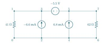
Although we've assigned node labels for all the nodes, we should note that nodes 1 and 2 are the same, as are nodes 5 and 7, as are nodes 0, 2, 4 and 6. Therefore, if we define node 2 as our reference, then we can determine all the voltages in this circuit by solving for the voltages at nodes 3 and 5, which are shown in red in the following circuit diagram:
