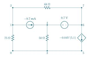
As with previous examples, we've labeled all of the circuit's nodes, but if we select nodes 0, 3 and 5 as the reference (or ground), then we can solve for all of the voltages in this circuit by finding the voltages at nodes 1, 4 and 6:
