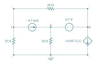
The dependent current source between nodes 6 and 5 is controlled by the voltage drop from node 5 to node 1, but because node 5 is our reference, we can write
