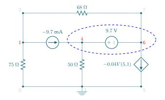
and then apply KCL to that region, noting that  $V_4 = V_6 + 9.7$ :
