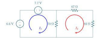
we move around the loop in a clockwise direction, add all of the voltage drops, then set the sum equal to zero:
