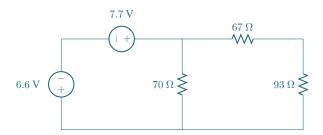
To apply the mesh-current method to this circuit, we first identify loops within the circuit. A loop is simply a closed path through the circuit that originates and ends at the same point. Two possible loops in this circuit are shown below:
