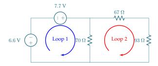
Loop 1 traverses clockwise through the 6.6 V source, the 7.7 V source, and the 70  $\Omega$  resistor; whereas Loop 2 traverses clockwise through the 70  $\Omega$  resistor, the 67  $\Omega$  resistor, and the 93  $\Omega$  resistor. We might also define a loop through the 6.6 V source, the 7.7 V source, the 67  $\Omega$  resistor, and the 93  $\Omega$  resistor, but, as we will see below, this loop would be redundant for the purposes of applying the mesh-current method.
