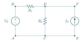
Because of the current source in parallel with the  $R_2$  resistor, you CANNOT use the voltage division method in this way:
