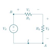
The voltage drop across the two resistors is equal to the voltage drop from node *B* to node *A*, which is equal to the source voltage:
