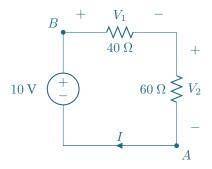
The voltage across the 40  $\Omega$  resistor is:
