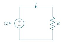
Because the positive and negative terminals of the voltage source are connected directly across the resistor, the voltage across the resistor is 12 V. The direction for the current that is labeled *I* is such that it enters the resistor on the side with the positive polarity and exits on the side with the negative polarity. Accordingly, we can use Ohm's Law to relate the voltage and current as:
