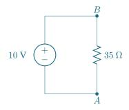
Here, we have replaced the two 20  $\Omega$  resistors, the 30  $\Omega$  resistor, and the 70  $\Omega$  resistor with an equivalent resistance of 35  $\Omega$ . Using this simple circuit, we could determine that the current flowing from the 10 V source is
