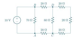
Note that the three resistors on the right side of the circuit can be combined in series to form an equivalent resistance equal to  $20 + 20 + 20 = 60 \Omega$ . That equivalent resistor is in parallel with the  $60 \Omega$  resistor between nodes *C* and *D*, so, if we combine those we can replace the four resistors with an equivalent resistance determined by
