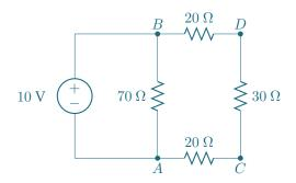
Now we can combine the three resistors on the right of the new circuit to form an equivalent resistance equal to  $20 + 30 + 20 = 70 \Omega$ . This equivalent resistor is in parallel with the 70  $\Omega$  resistor
