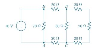
For the purpose of analyzing the currents and voltages to the left of nodes *C* and *D*, we could replace the circuit with this one:
