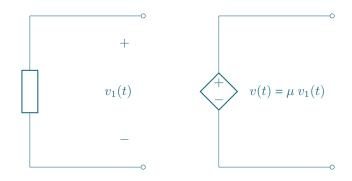
If, for instance,  $\mu$  is equal to 4 and  $v_1(t)$  is equal to 3 V, then the voltage across the source would be  $4 \times 3 \text{ V} = 12 \text{ V}$ .
