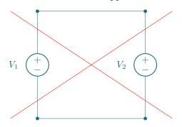
That is, you should not connect a voltage source in *parallel* with another. You should immediately question this configuration if you encounter it in a circuit diagram. Think about how confusing this would be, for instance, if  $V_1 = 5$  V and  $V_2 = 10$  V. The voltage across the two sources would have to be equal to both 5 V and 10 V.
