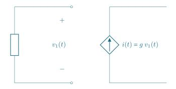
Again, we use a diamond instead of a circle for the source symbol, and the arrow shows the reference direction for the current. As we've shown here, in most situations the current will be proportional to the controlling voltage. In this case, the proportionality factor is g, where g has units of amps per volt.
