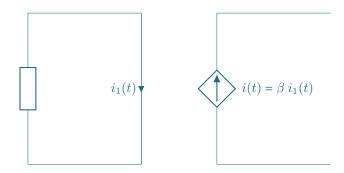
For this example, the current supplied by the source is proportional to some controlling current with a proportionality constant equal to  $\beta$ .
