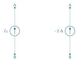
For the second source, a current of -2 A flows from terminal **B** to **A**, or, equivalently, a current of +2 A flows from terminal **A** to **B**.
