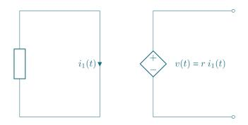
For a voltage-controlled voltage source, the proportionality constant is unitless. For a current-controlled voltage source, the proportionality constant has units equal to volts per amp.
